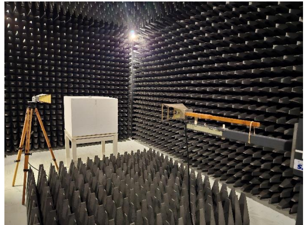
Figures 8 & 9: Measurement Setup for Radiated Emissions between 30 MHz and 4 GHz
