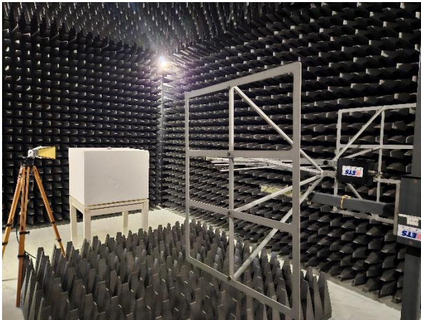
Figures 8 & 9: Measurement Setup for Radiated Emissions between 30 MHz and 4 GHz
