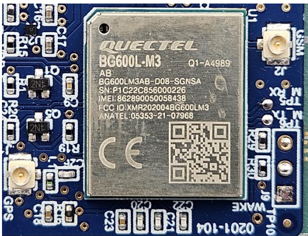
Figures 14 & 15: Detailed View of RF Circuit and Antenna
