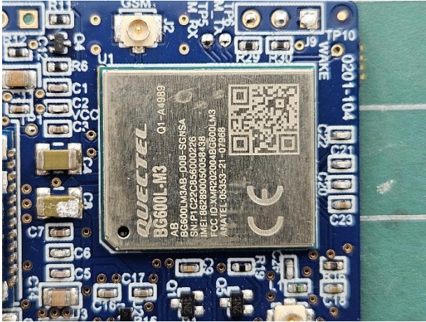
Figures 12 & 13: Detailed View of RF Circuit and Antenna
