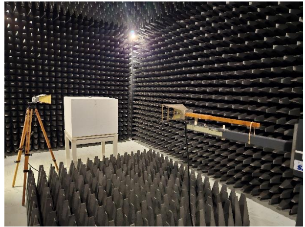
Figures 6 & 7: Measurement Setup for Radiated Emissions between 30 MHz and 8.3 GHz
