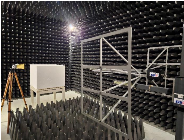
Figures 6 & 7: Measurement Setup for Radiated Emissions between 30 MHz and 8.3 GHz
